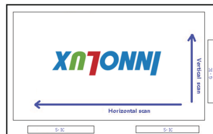
Fig. 2 Reverse scan (Pin24, Reverse = High)
