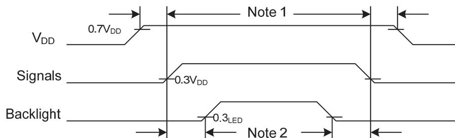
Note 1: In order to avoid any damages,  $V_{DD}$  has to be applied before all other signals. The opposite is true for power off where  $V_{DD}$  has to be remained on until all other signals have been switch off. The recommended time period is 1 second.
