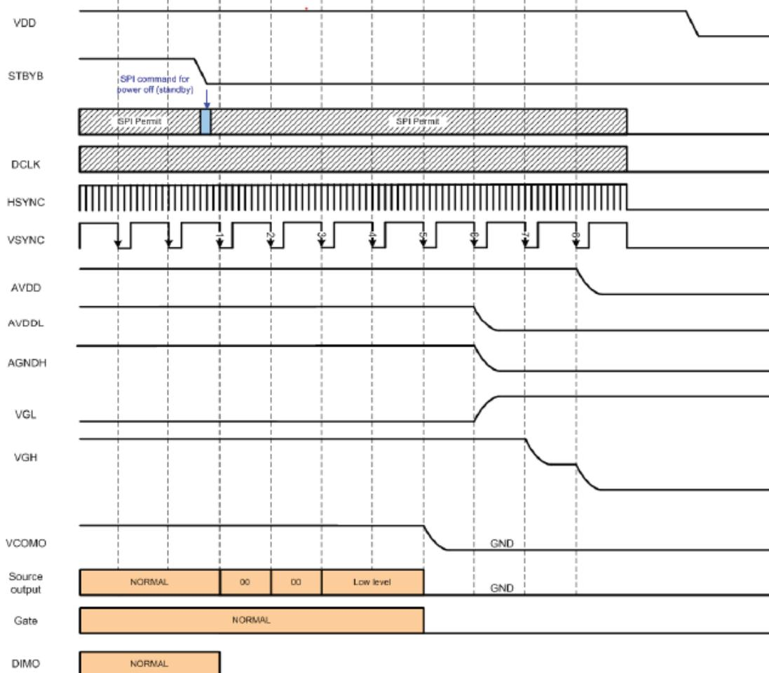
**Figure 8.2: Power off timing sequence**
