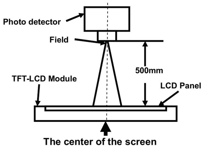
Note 2: Definition of viewing angle range and measurement system.
