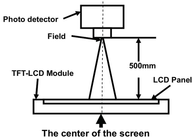
Note 2: Definition of viewing angle range and measurement system.
