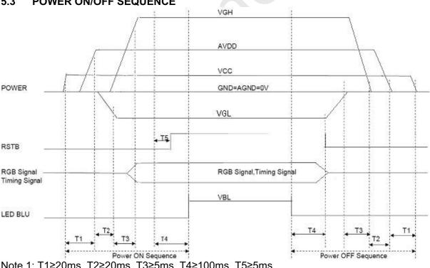
Note 1: T1≥20ms, T2≥20ms, T3≥5ms, T4≥100ms, T5≥5ms.
