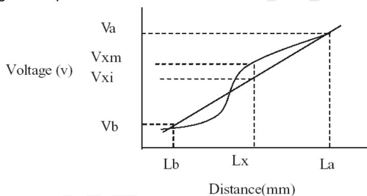
$$\text{Linearity} = \frac{|V_{xi} - V_{xm}|}{(V_a - V_b)} * 100\%$$
