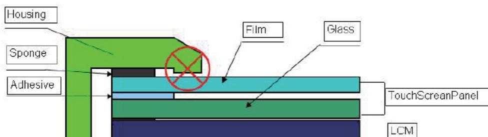
3. Use a buffer material(Gasket) between the TSP and housing to protect damage and wrong operating
