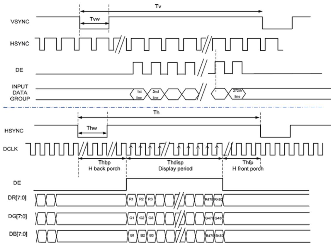
Figure 6.4.1 Data Input Timing Diagram Under SYNC-DE Mode
