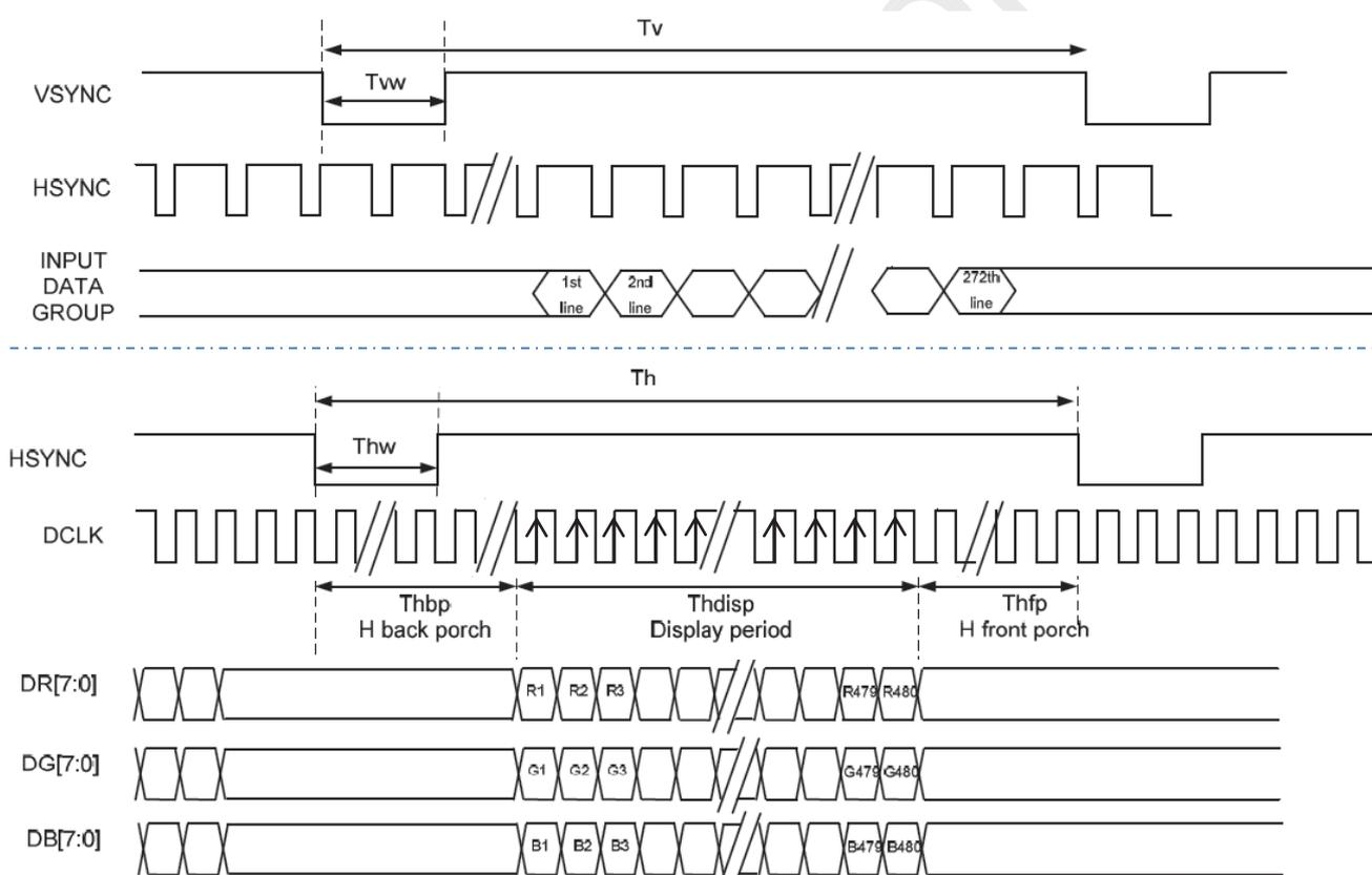
Figure 6.3.1 Data Input Timing Diagram Under SYNC Mode
