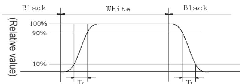
Fig4. Response Time Testing(SFT)
