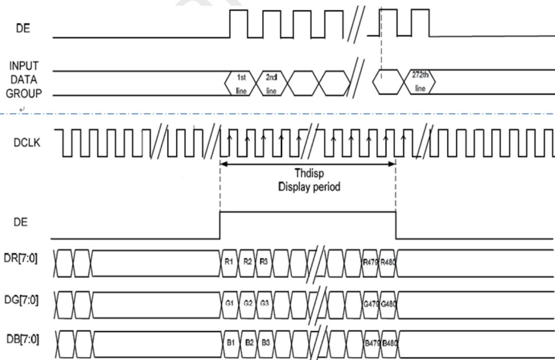
Figure 6.5.1 Data Input Timing Diagram Under DE Mode
