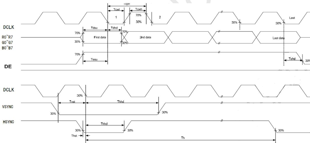
Figure 6.1.1 Clock and Data Input Timing Diagram
