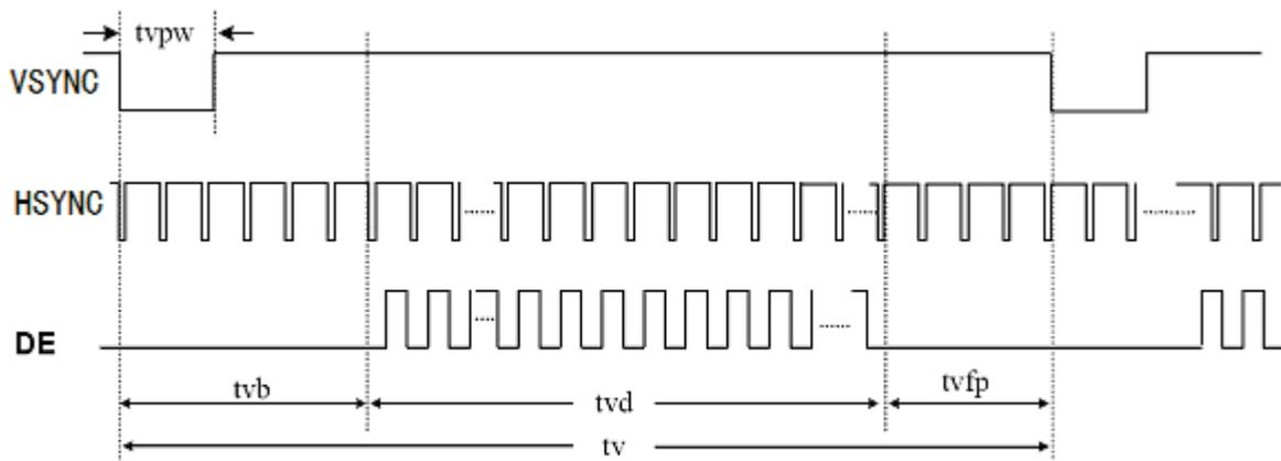
Figure 6.3.1 TCON Vertical Input Timing Diagram HV
