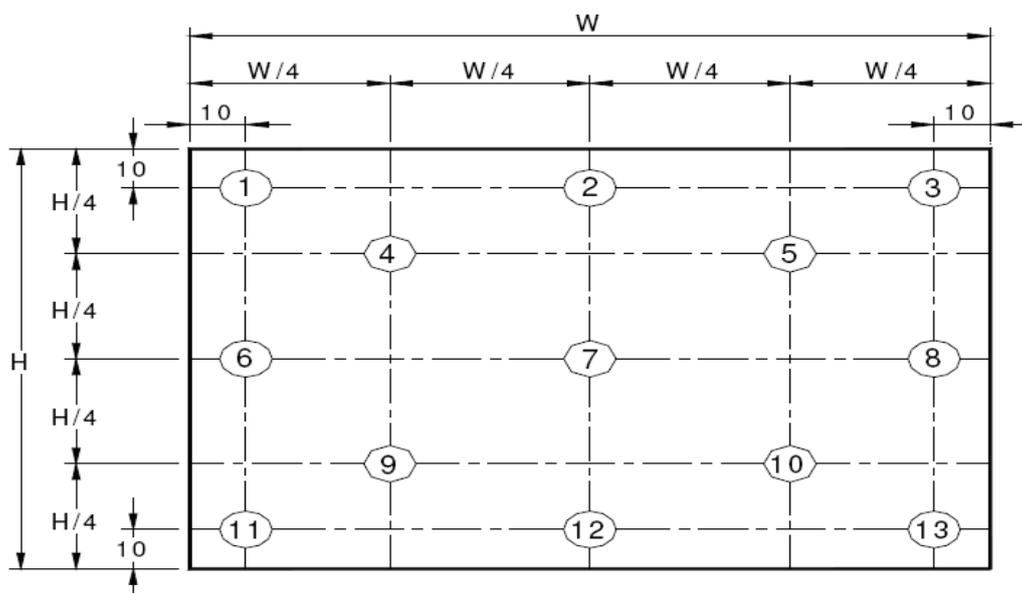
The White luminance uniformity on LCD surface is then expressed as :  $\Delta Y_5 = \text{Minimum Luminance of five points} / \text{Maximum Luminance of five points}$  (see FIGURE 2) ,  $\Delta Y_{13} = \text{Minimum Luminance of 13 points} / \text{Maximum Luminance of 13 points}$  (see FIGURE 3).
