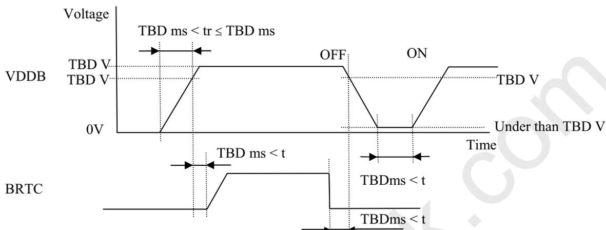
Note1: The backlight should be turned on within the valid period of LVDS signals, in order to avoid unstable data display.
