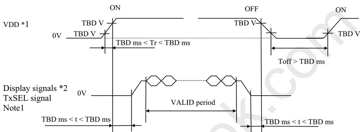
\*1 In terms of voltage variation (voltage drop) while VDD rising edge is below TBD V, a protection circuit may work, and then this product may not work.
