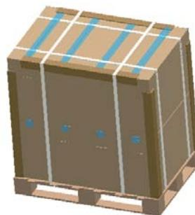
**4.-Put the Pallet into Truck with 2 rows and 2 layers**
