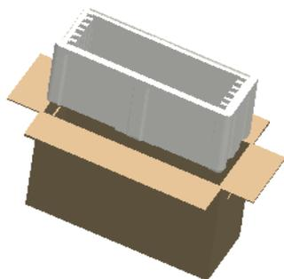
**2.-Put Protection Film on Panel , Put MDL in PE Bag**
