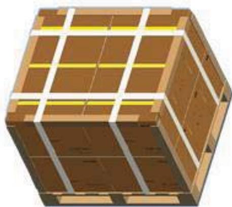
Put totally 12 boxes. Place paper corners and wrap film around the boxes. Pack with 4 packing belts.
