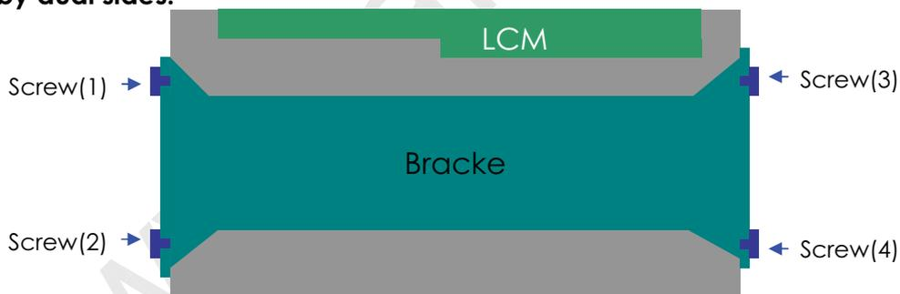
9.5 The system bracket and panel should be in parallel with having no gap after inserting screws.
