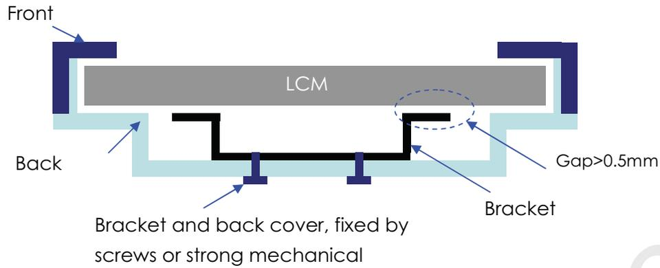
9.3 The EMI gasket should be uniform and not push panel strongly.
