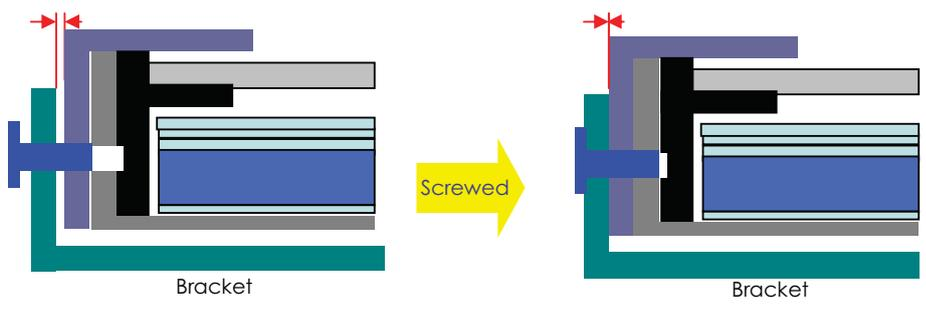
**9.6 Avoid scratching LCM, the rib on system front-cover should not exceed the bottom edge of LCM's front-bezel.**
