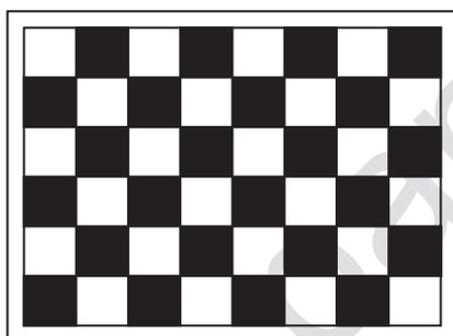
**Typical power Pattern**
