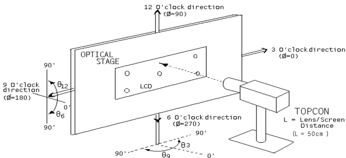
Figure 2. White Luminance and Uniformity Measurement Locations (9 points)
