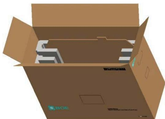
Place the modules bundled by packing bag in the box, 8pcs module per box, place a cover on the top of the box
