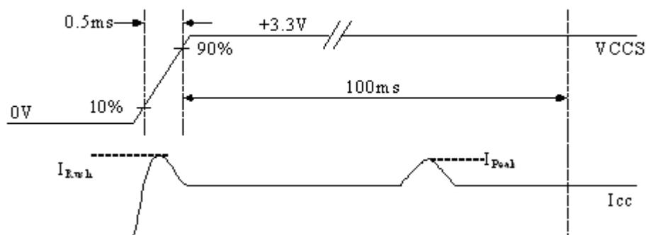
Note (3) The specified power supply current is under the conditions at VCCS = 3.3 V,  $T_a = 25 \pm 2^\circ\text{C}$ , DC Current and  $f_v = 60\text{ Hz}$ , whereas a power dissipation check pattern below is displayed.
