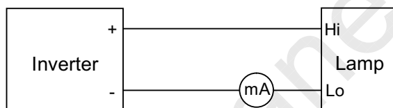
(Figure. 1: Measurement of return current)
