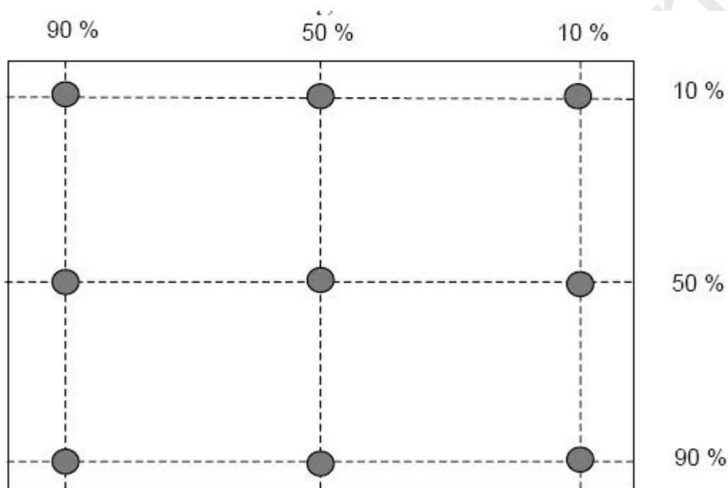
The White luminance uniformity on LCD surface is then expressed as :  $\Delta Y9 = \text{Minimum Luminance of five points} / \text{Maximum Luminance of 9 points}$
