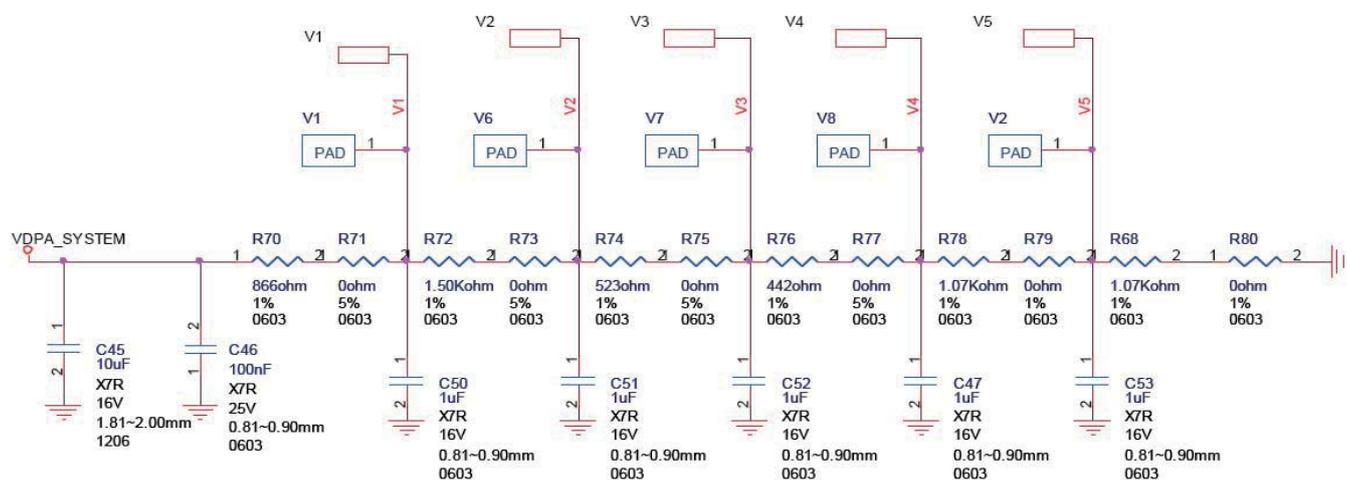
Gamma & Vcom : Generate by VDNA\_SYSTEM and VDPA\_SYSTEM
